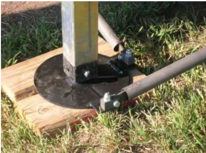
Excel - They welded tabs on the footplate, but it is simpler to just weld the bolts to the footplate.
