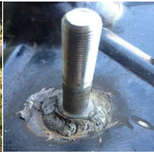
Excel - They welded tabs on the footplate, but it is simpler to just weld the bolts to the footplate.
